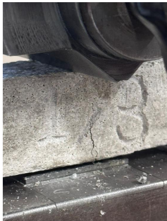
Figure 3. Tensile test strength using flexural loading
