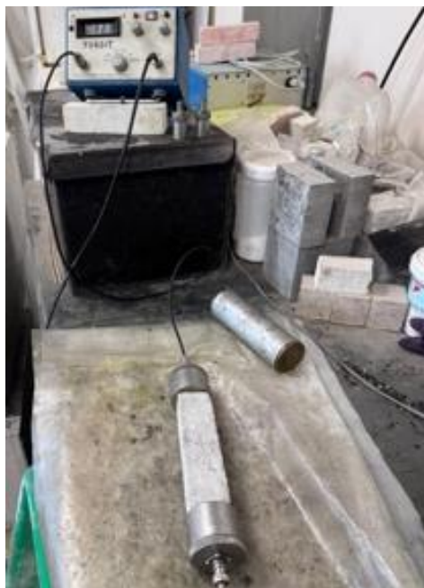
Figure 4. Ultrasonic pulse velocity test illustration
