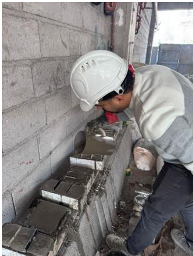
Figure 1. Pouring the FC into molds.
